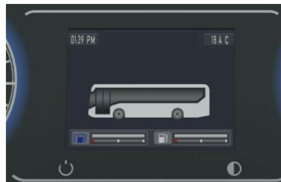
Stop mode - This is displayed with the hand-brake applied. In addition to driving mode, a bus is depicted. Doors will turn black if open.
