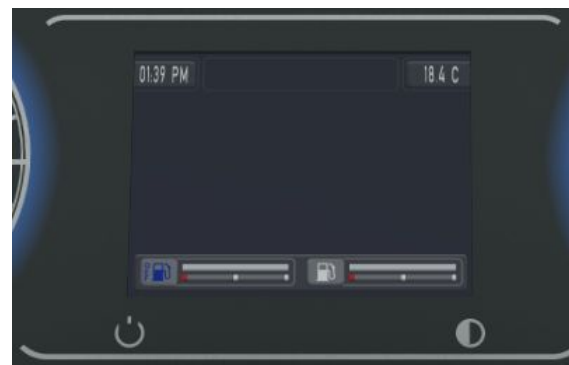
Driving mode - This is displayed when the handbrake is not applied. Current time (top left), Saloon temperature (Top right), Fuel gauge (Bottom left), DEF level (Bottom right (Not used))
